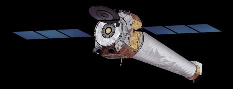
NASA's Chandra X-ray Observatory, which was launched by the Space Shuttle on July 23, 1999, is a telescope specially designed to detect X-ray emission from very hot regions of the Universe such as exploded stars, clusters of galaxies, and matter around black holes. Because X-rays are absorbed by Earth's atmosphere, Chandra must orbit above it, up to an altitude of 139,000 km (86,500 mi) in space.
