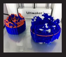
Select the 3D printer of your choice. For this example (shown left) two colors were used, and support structures were manually removed. The remaining parts of the ring are clearly visible in red in the print on the right. Using the Ultimaker 2 printer this model took about ten hours to print.
